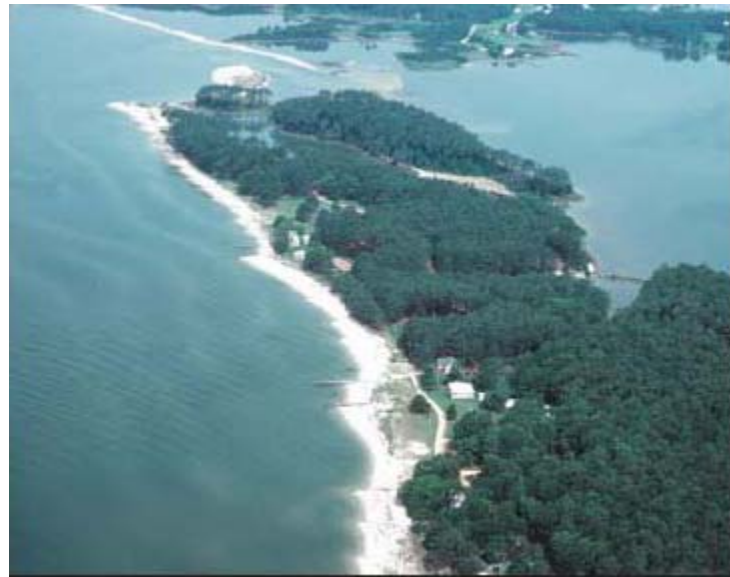
Figure I-6: Shoreline along the Rappahannock River, Virginia as a result of groin construction
