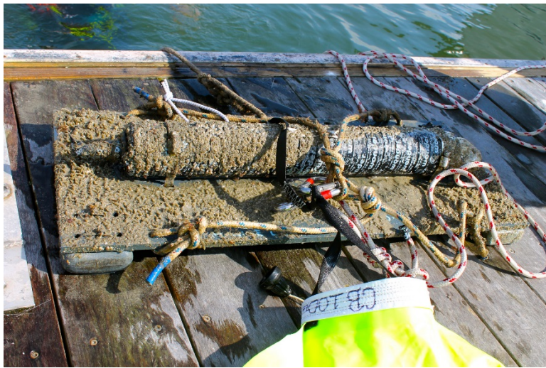
Figure 2. An Aquadopp Current Profiler mounted upon a base after retrieval. The sensors are at the head of the instrument (right).
