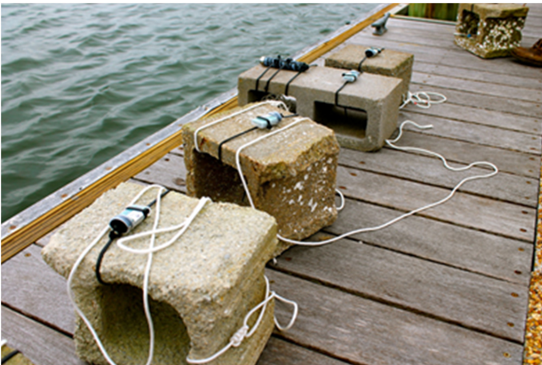
Figure 2. Design for light sensor experiment for the bottom of the yacht basin.
