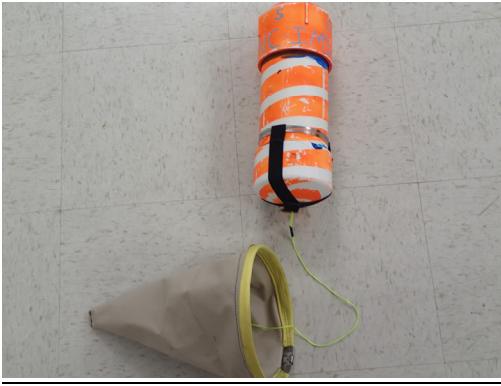
Figure 3. A drifter and attached drogue. The PVC housing capsule (orange and white cylinder) is tethered to a conical drogue made of durable and flexible plastic.
